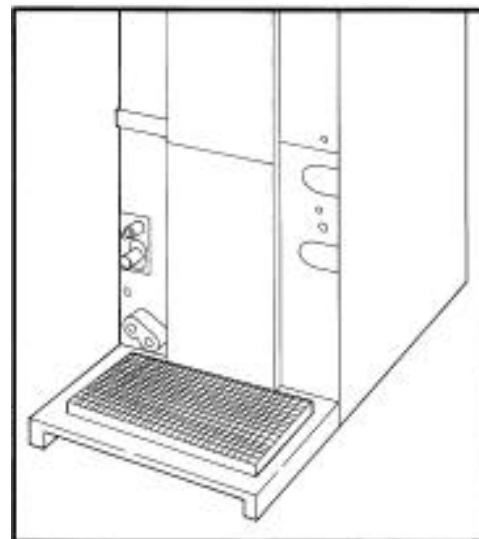
Fig. 4—Removing Filter from Fan Coil Unit
